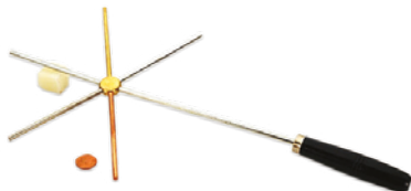
Instrument for demonstrating the thermal conductivity (expansion) of different metals
